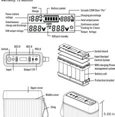
INPUT (Charging port 7.9\*5.5mm): 13-25V 65W@ Wall charger, 5.5 hrs 18V 50W @Solar Panel, 3.7-6 hrs
