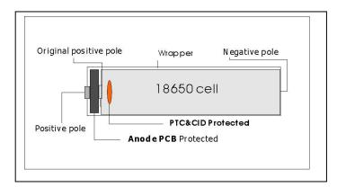
2 Polymer Li-ion Battery Pack Characteristics
